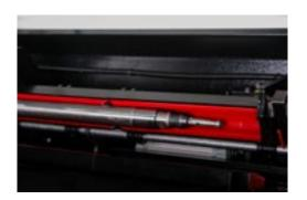
Thanks to the collet type system, the channel can be adjusted according to the max. material diameter and it allows you to work with a single channel without need a replacement. The remnant retracts into the bar feeder and falls into bin.
