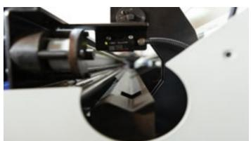
the length of bar can not be longer than spindle length
